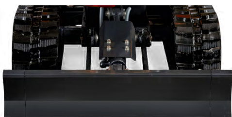
Extended undercarriage 840 mm - Increased stability
