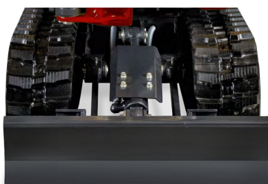
Retracted undercarriage 680 mm - Best manoeuvrability
