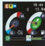
PM accumulation/ Urea accumulation display
