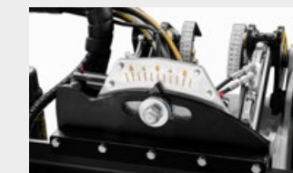
Hydraulic tilt for direct control from the cab
